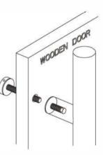
D: Single fixing on wooden doors with cover caps Bolt-through fixing, for door thickness 35-55mm
